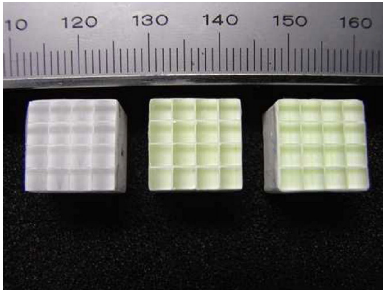
Fig. 7. Pictures of the 4 \times 4 scintillator matrices to be coupled with the MPPC array. (From left to right: Ce:LYSO, Pr:LuAG, Pr:LuAG (WLS)).
