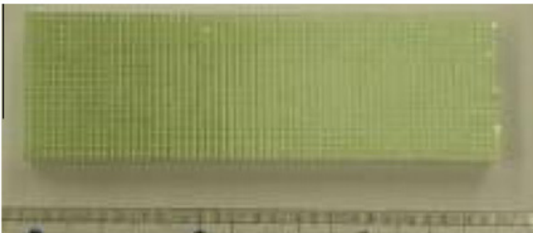
Fig. 3. The 20 × 64 Pr:LuAG pixelated array for Pr:LuAG-PEM.
