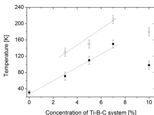
The temperature of separation and the temperature of maximum of magnetization measured in ZFC modes versus concentration of Ti-B-C system in 316L austenitic steel in a magnetic field of 100 Oe, empty and full circles, respectively. Involving the superparamagnetic model, we can interpret not only the low-field dependence of the ZFC and FC magnetization, but also a linear change of  $T_{max}$  and  $T_{ir}$  with increasing dopant concentrations up to 7 vol. %
